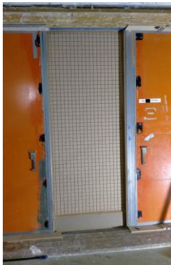
Figure 7 50x50mm routed slots in a panel mounted for diffuse field testing
