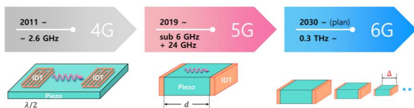
Figure 2 A schematic diagram of (a) a SAW filter (b) a BAW filter (c) Size of BAW filter getting smaller in response to higher frequencies
